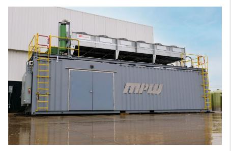
MPW'S COMPRESSED AIR SOLUTION ELIMINATES LARGE CAPITAL EXPENDITURES MPW Industrial Air Utility Services offers energy-efficient Ingersoll Rand centrifugal, oil-free compressors designed to meet customers' Compressed Air Solution (CAS) needs. These compressors, available with air-cooled or integrated cooling systems, are packaged in plug-and-play modules that are easily transportable and continuously monitored by MPW.
