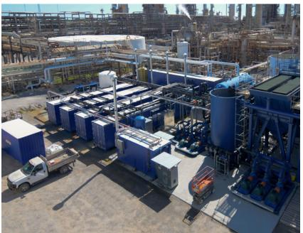
MPW'S CUSTOM INDUSTRIAL AIR SERVICES PROVIDE TURNKEY SOLUTIONS MPW Industrial Air Services (IAS) builds unitized, energy-saving compressed air modules to customer requirements, replacing the need for customers to own, operate, maintain or monitor facility compressed air needs.
