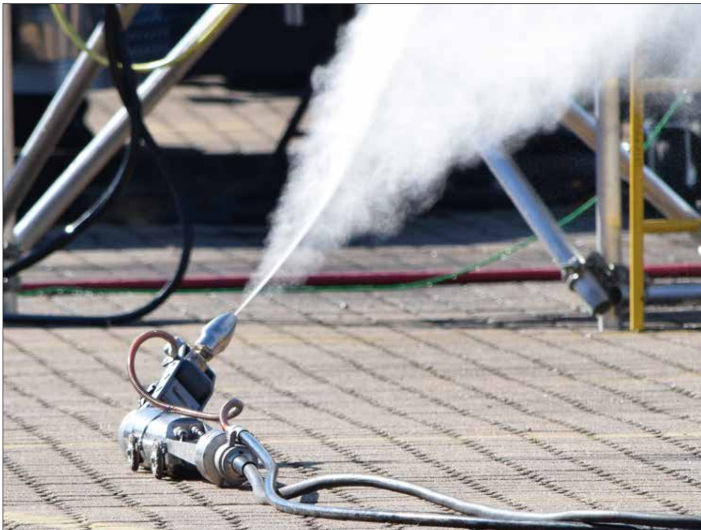
IDTec USA demonstrates its precision waterjet cutting module and transporter, which uses low volume and high pressure to precisely remove deposits from within 6-inch to 15-inch pipes without damaging the pipe. The device is capable of removing root balls, hardened fat, grease, cement, scale, calcium and mineral build-up. The live demonstration was held during the 2017 WJTA-IMCA Conference & Expo.
