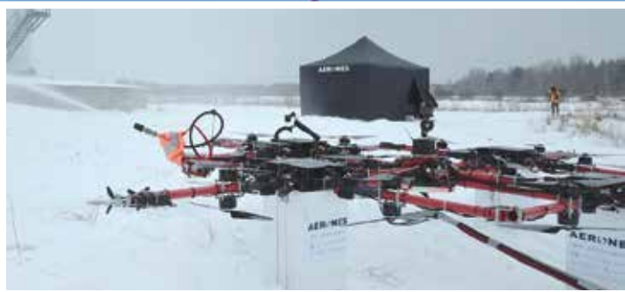
Aerones' UAVs are tethered to water and electric supply on the ground.
