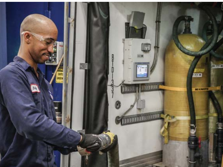
A technician prepares a demineralization trailer for dispatch to a customer site.
