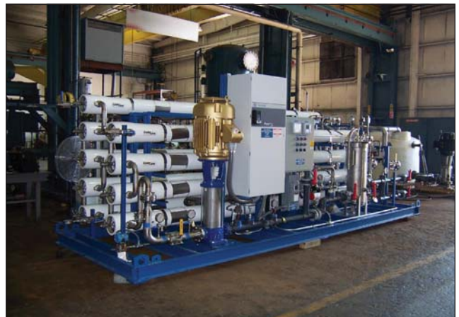
The demineralization trailers feature a capacity of 10 million grains.
